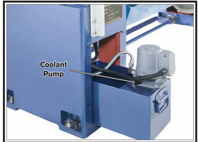
Figure 141. Coolant pump location.
